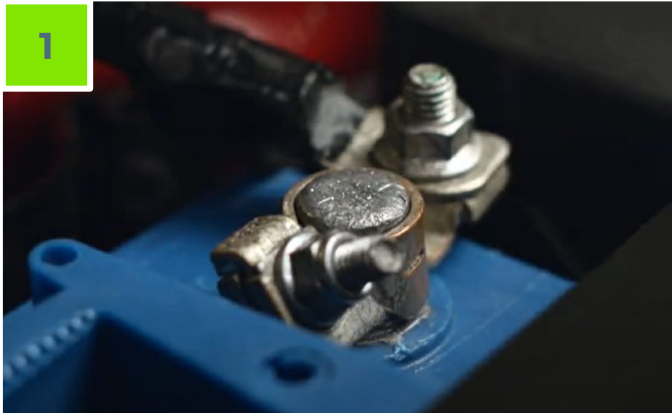
Step 1. Disconnect the negative battery cable.
