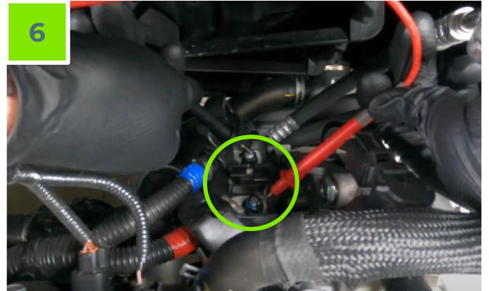
STEP 6 - Check with the multimeter the absence of current in the iBSG
