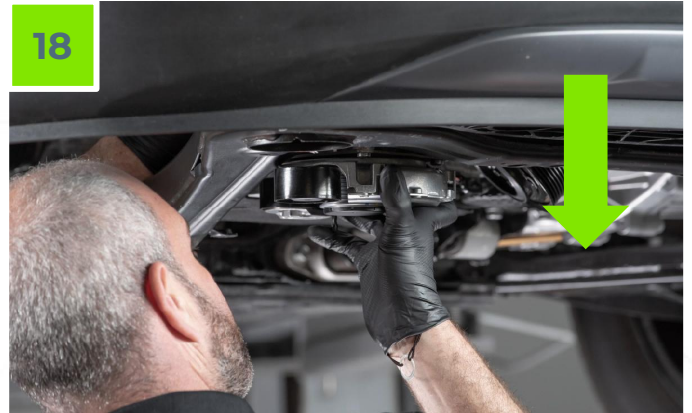
STEP 18 - Rotate the iBSG & take it out with the regulator part down
