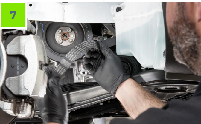
STEP 7 - Place the belt in the correct position defined by the car maker (it's recommended to install a new one)
