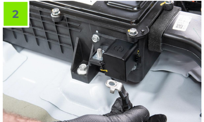
STEP 2 - Disconnect +12V terminal in 48V pack
