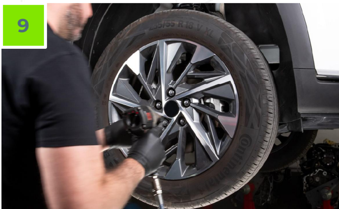
STEP 9 - Remove the wheel
