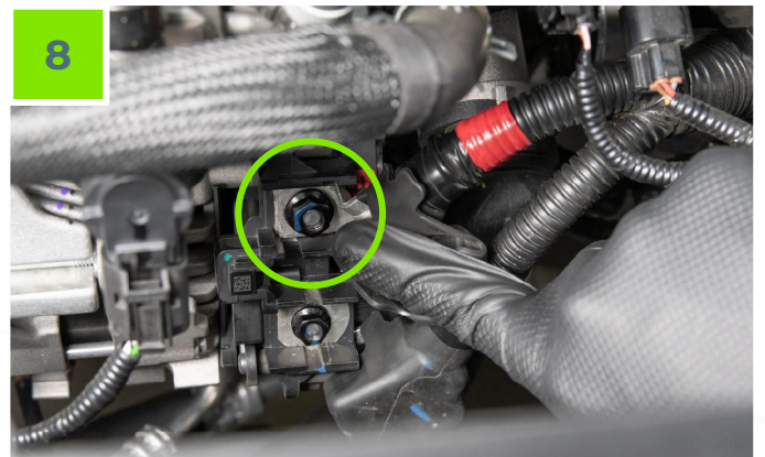
STEP 8 - Disconnect +48V terminal from the iBSG
