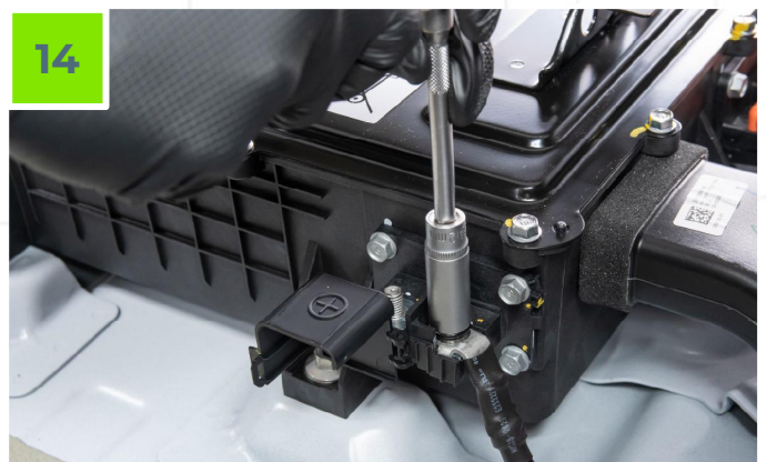
STEP 14 - Plug again +12V terminal in 48V pack
